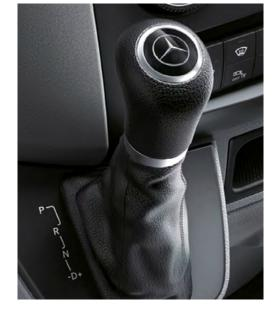
As before, the gearshift (gate-type gearshift P, R, N, D) for the 7G-TRONIC PLUS automatic transmission is integrated in a center console built into the vehicle interior.
