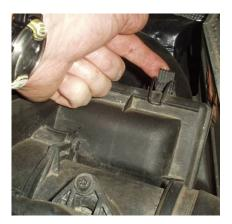
Two plastic spring tensioner tabs are located at the back of the air filter housing. Release the tabs.
