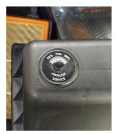
DC offers as an option an air flow indicator to inform owners of when to change the air filter. It is located on the top left of the air filter canister. Even though my old filter (the lower one in the picture above) appeared to be dirty and had 28,000 miles on it, the air flow indicator showed no problem. So what to believe? Other members of the Yahoo Sprinter Group also report bafflement as to whether this feature works.
